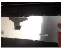
Pick up the keyboard and disconnect the flex cable.
