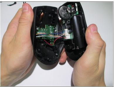
Pry the center of the mouse apart to separate the upper and lower housing of the boards.
