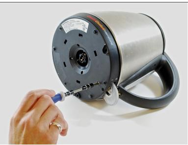
Remove the five 3/8" screws from the base of the kettle using a Phillips #1 screwdriver.
