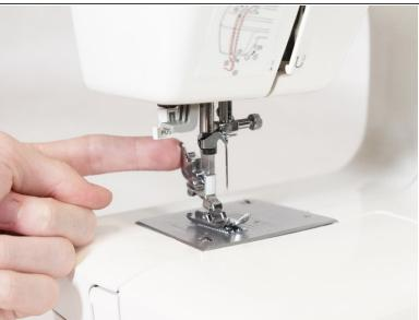
Lift the arm on the back of the presser foot assembly to release the foot.
