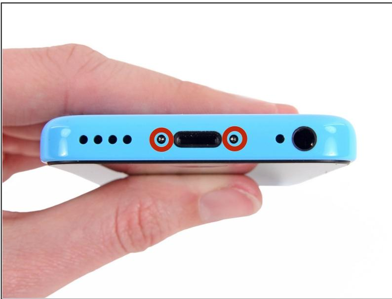
**⚠ Before you proceed, discharge your iPhone battery below 25%. A charged lithium-ion battery can catch fire and/or explode if accidentally punctured.**
