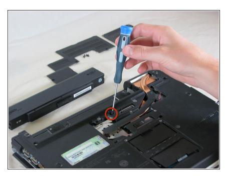
Using a Philips screw driver, unscrew the rear keyboard screw from the bottom of the laptop.
