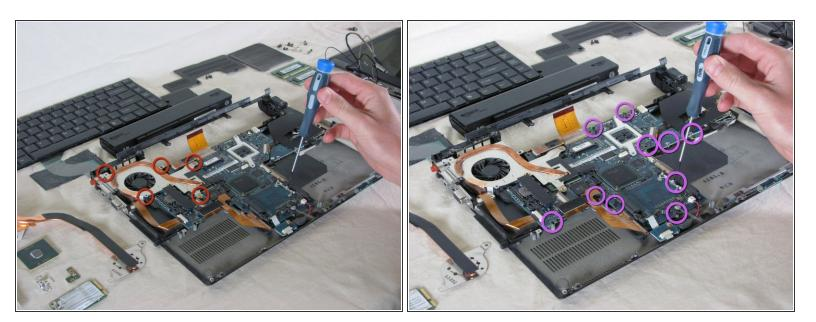
↑ Caution: When removing the fan, be careful to not tear the attached ribbon cable.
