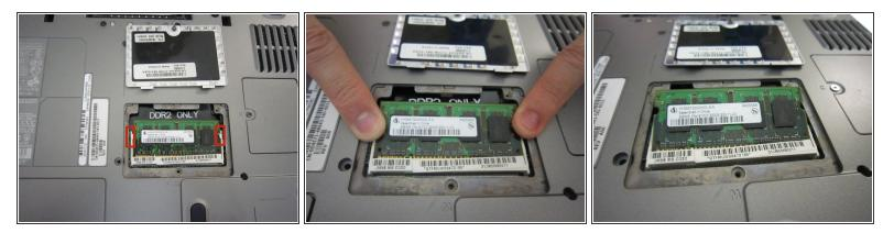
Using two fingers, push the silver ends away from the RAM until the RAM is released.
