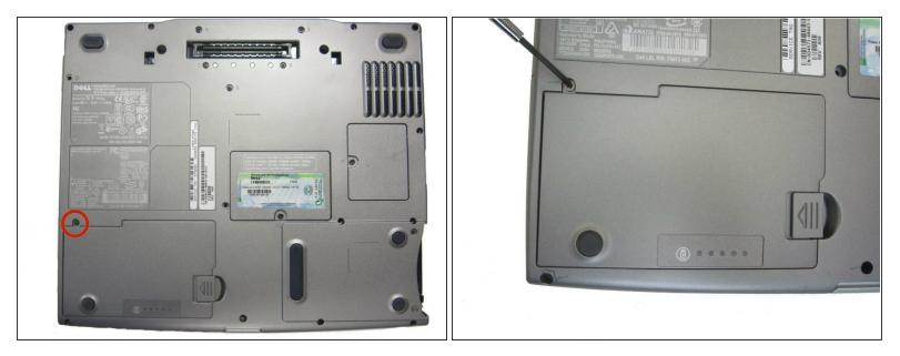
• Remove the 3.9 mm Phillips #1 screw from the battery compartment.
