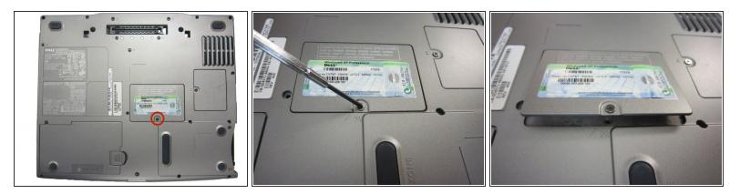
• Remove the 3.9mm Philips #1 screw holding the panel for the RAM.
