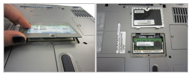
• Lift and remove the panel.
