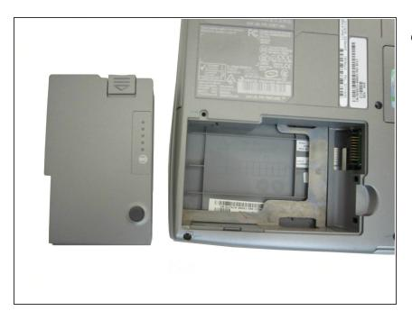
• Remove the battery from its compartment.
