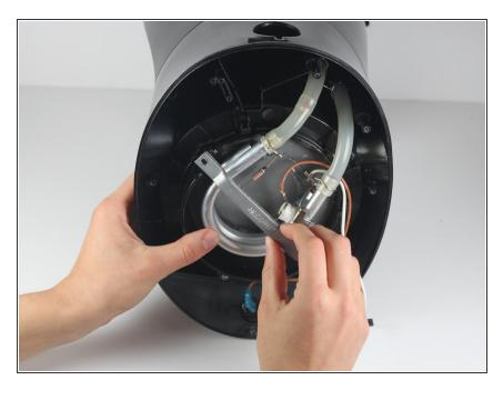
Gently lift the silver support bracket freeing the heating plate from the heating coil.
