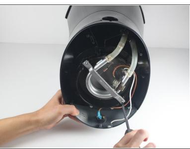
Identify and remove the two 13mm screws securing the silver support bracket using a phillips head screw driver.
