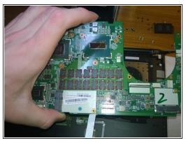
Removing the mainboard.
