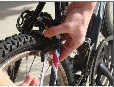
Locate and remove the dome nut with a 10mm open-end wrench.
