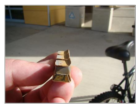
Inspect brake pad for wear.
