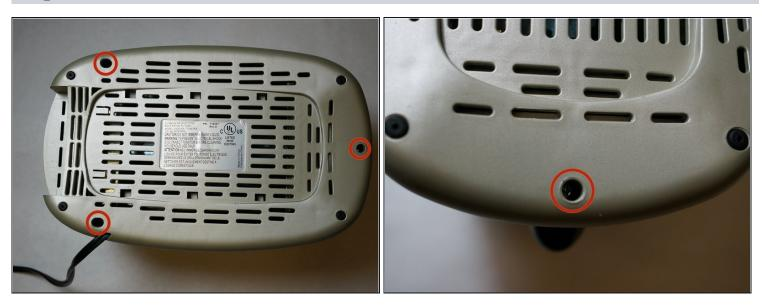
• Using the Phillips-head #2 screwdriver, unscrew the three 1cm Phillips-head screws on the plastic base of the toaster to separate the outer metal shell from the plastic base.
