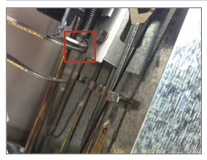
• Insert the <u>tweezers</u> between the spring and the bottom of the lever to release the spring.
