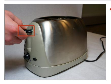
Push the plastic push-down handle down and pull the plastic handle straight from metal arm.
