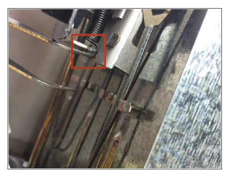
Insert the tweezers between the spring and the bottom of the lever to release the spring.
