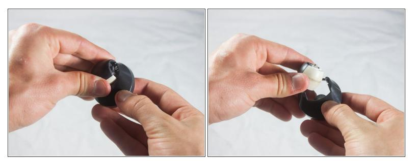
Firmly grasp the wheel, and pull to separate from the housing.
