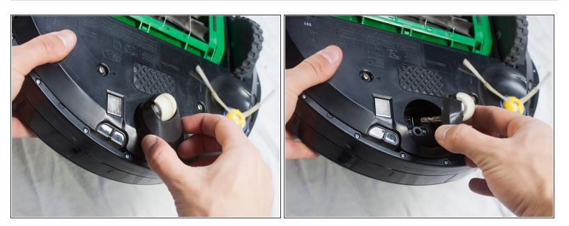
Grab the front wheel housing on the bottom of your Roomba and lift to remove.
