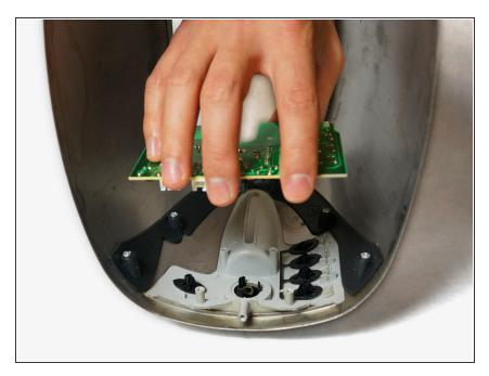
Grasp the circuit board and pull on it perpendicular to the attached surface.
