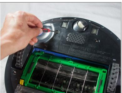
Using a Phillips #2 screwdriver, remove the captive screws that hold the bottom plate in place.
