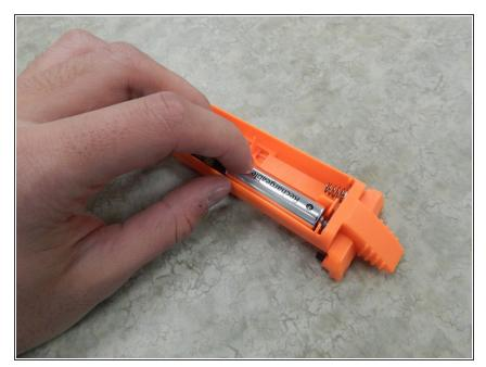
Apply downwards pressure on the battery you're trying to remove in the direction of the spring.
