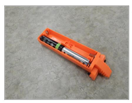
When installing new batteries, ensure that their polarities are facing the correct directions. Follow the inscriptions on the bottom of the battery tray, or place the flat side of each battery against the spring.
