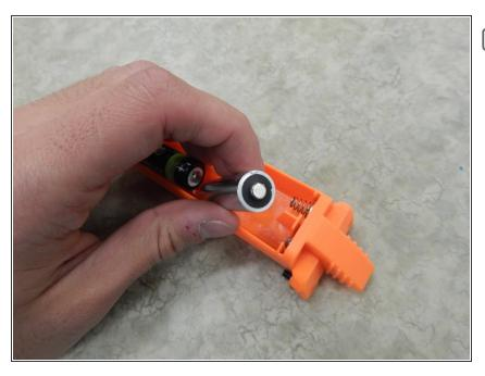
Pull battery straight out. Do not throw used batteries in the trash! Please electronically recycle them properly.
