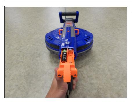
Pull the battery compartment out and away from the gun.
