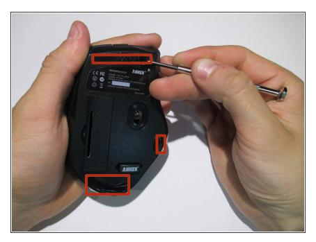
Peel off the stickers. This will reveal the location of four screws.
