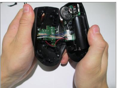
Use a spudger to pry apart the upper and lower housing of the mouse.
