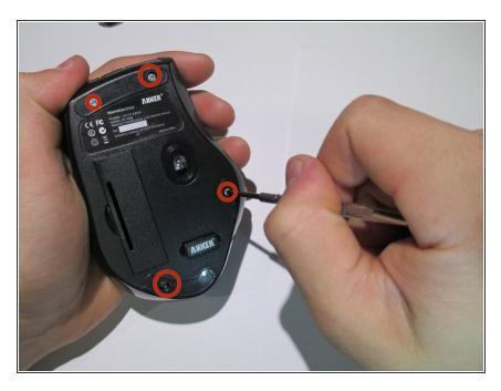
Remove the four screws using a Phillips #0 screwdriver.
