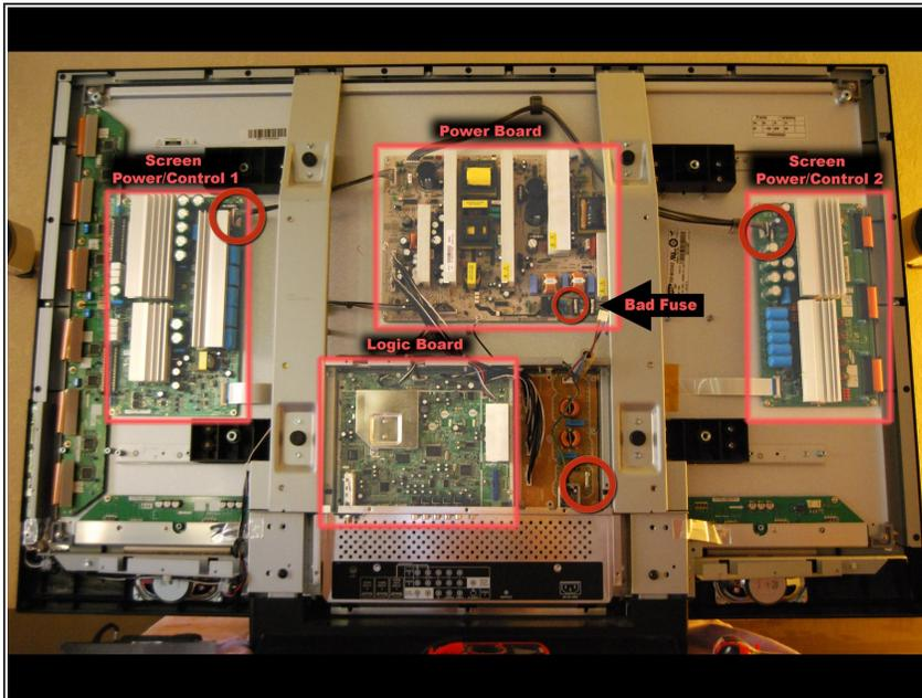
**⚠ Caution:** Before you remove the motherboard, be cautious of the many capacitors throughout that could cause serious injury. Use a discharge probe to safely rid the capacitors of dangerous charges.
