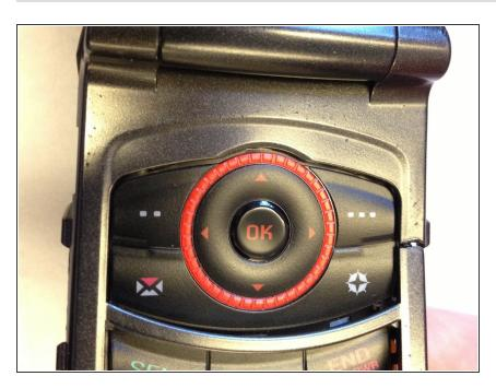
Check if the edges are perfectly aligned between the two plastic layers after you insert the keyboard.
