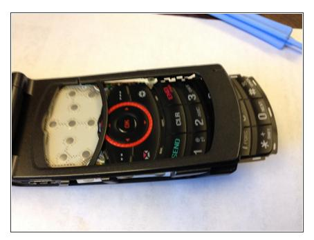
Slide out the keyboard carefully in between the two layers.
