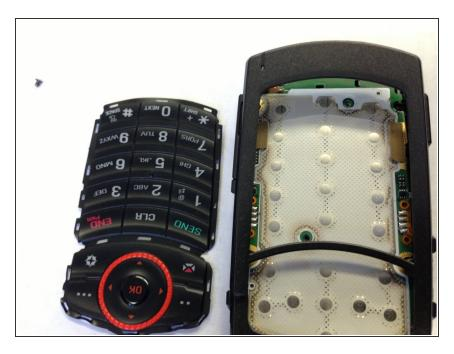
Insert the new keyboard in between the two layers carefully.
