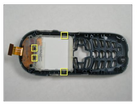
To remove the LCD screen, you will have to first release the 4 tabs that hold the screen in place.
