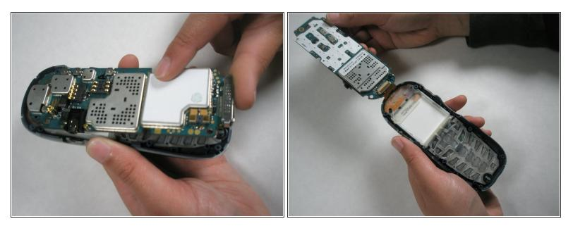
Place your thumb at the bottom of the logic board. Carefully lift up with your thumb to lift the logic board out of the casing.
