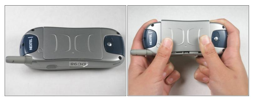
Press thumb against the top of the rear casing as shown and push down as you slide the casing off of the body.
