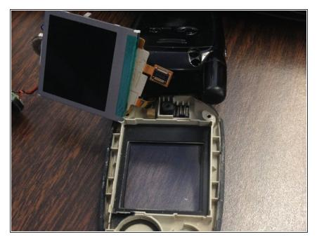
Carefully remove the screen from its holding frame.
