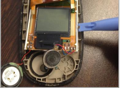
Detach the round magnetic batteries from their circular frames using an iFixit opening tool.
