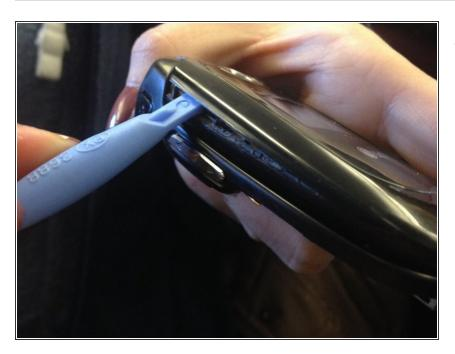
Remove the faceplate of the phone using an iFixit opening tool.
