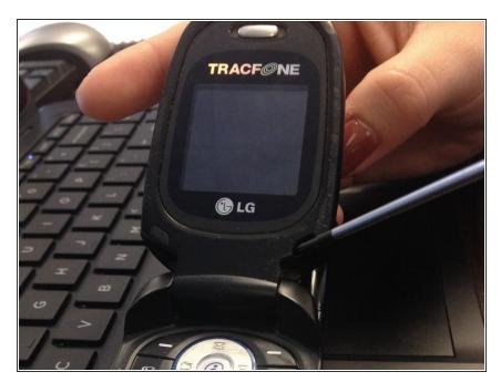
Use a spudger to pry out the rubber screw covers from the back and inside of the phone.
