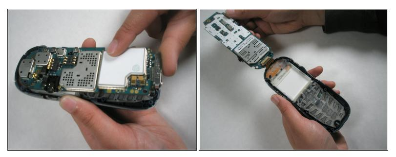
Place your thumb at the bottom of the logic board. Carefully lift up with your thumb to lift the logic board out of the casing.
