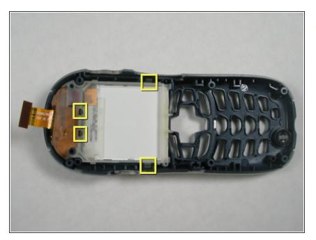
To remove the LCD screen, you will have to first release the 4 tabs that hold the screen in place.
