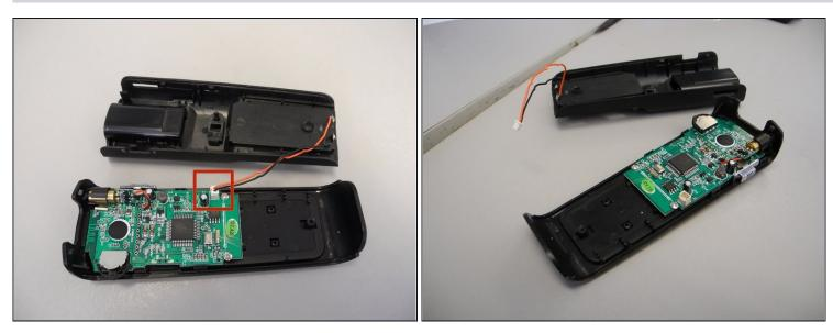
$\triangle$  There is a wire connector linking the front and the back of the device.
