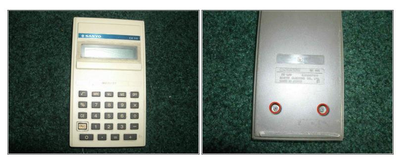
Remove these two screws from the back of the calculator using a Phillips #0 Screwdriver.
