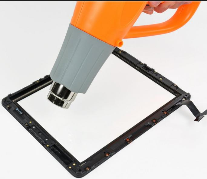
**⚠** In the following steps you will use a heat gun to soften the adhesive securing the black plastic frame to the front glass. Do not allow the stream of hot air to contact the thin rubber strip around the outer perimeter of the front glass as it may melt, permanently deform, and lose texture.
