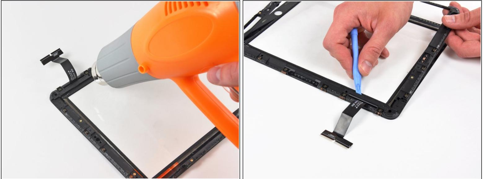
**⚠** In this step, you will heat and remove the plastic frame near the digitizer cable. Do not directly heat this ribbon cable, as it is extremely thin and sensitive to heat.
