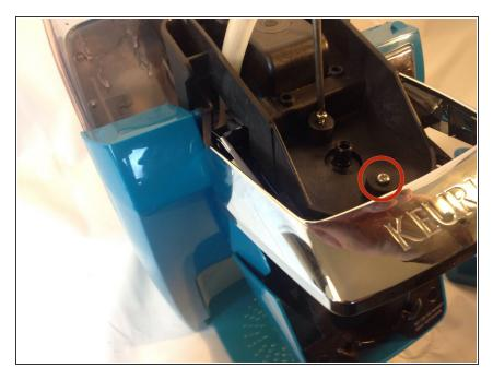
Unscrew the two 9 mm #1 Philips screws at the top of the device.
