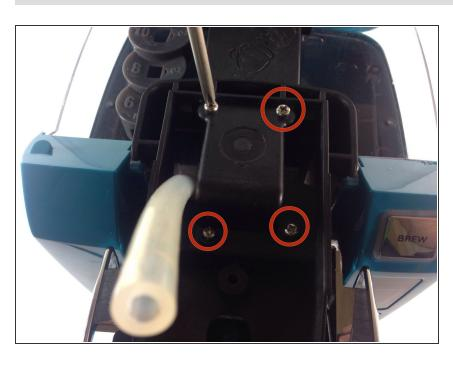
Use a Phillips #1 screw driver to remove the four 12 mm screws that hold the arm assembly in place.
