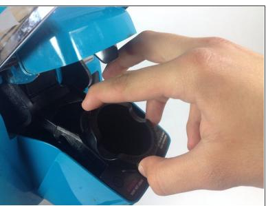
Firmly rock the K-cup holder from side to side, loosening the K-cup holder from its seat.
