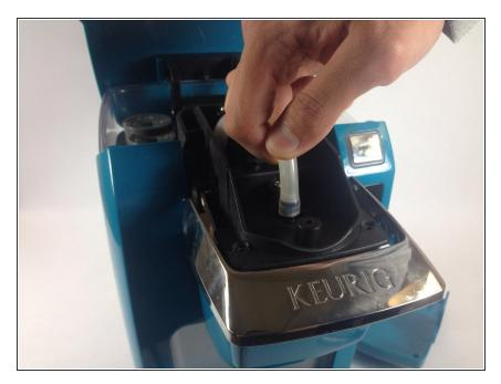
Firmly grasp the hose and pull it off of the plastic nozzle.
