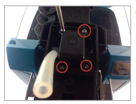
Use a Phillips #1 screw driver to remove the four 12 mm screws that hold the arm assembly in place.
