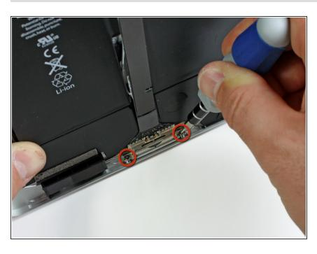
Remove the two 2.84 mm T5 Torx screws securing the dock connector cable to the rear panel assembly.
