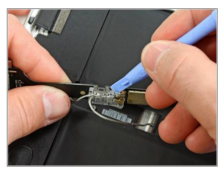
Carefully remove the plastic cover over the WiFi/Bluetooth board and dock connector cable using a plastic opening tool.
