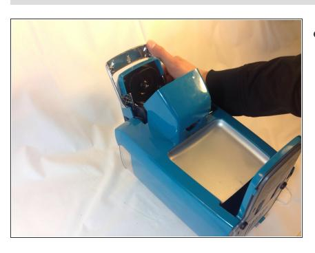
Lay the Keurig on its back with the water reservoir pointing away from you.
