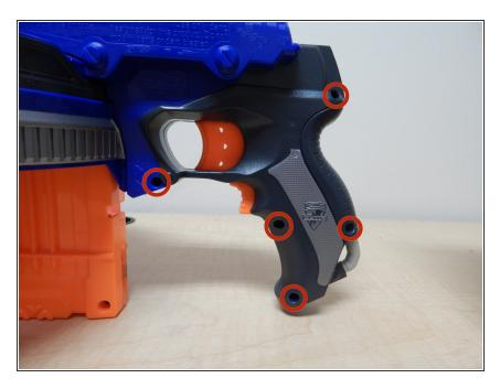
Remove the five 9.0 mm Phillips screws securing the trigger.
