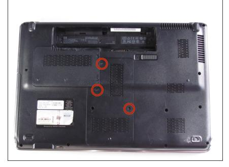
Using the Phillips #1, loosen the three 7mm captive screws that secure the memory module cover to the computer.
