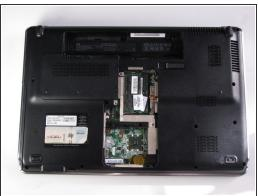
Remove cover and expose the memory module by lifting the cover up like its on a hinge.
