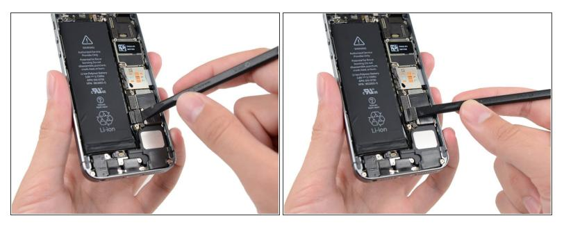
Use the flat end of a spudger to gently pry the battery connector up from its socket on the logic board.
