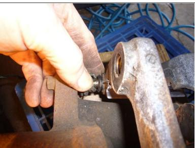
• If the carrier can't move freely back and forth, uneven pad wear can result. The pads should come with a tiny tube of high temperature grease. Carefully ease back the boots from the slides, and grease both rails. There's 2 for each side of the car, so budget accordingly.
