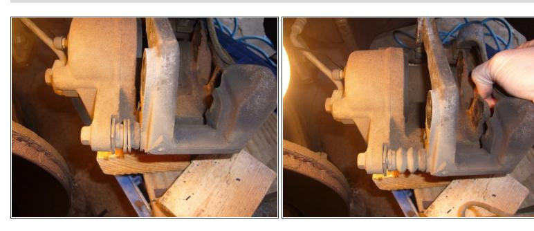
The pads ride in a carrier that's free to move in and out. These two shots show fully IN, and fully OUT. We will later have to grease these slides.
