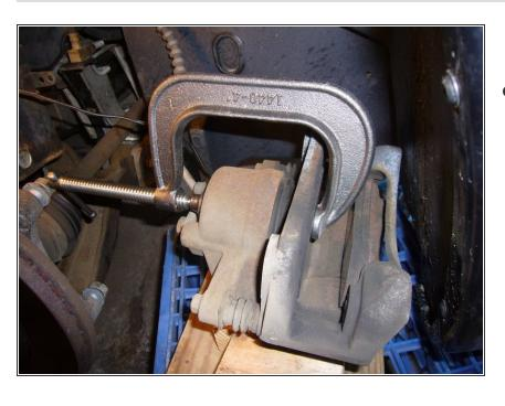
The new pads are thicker than the old, so the piston will have to be pushed back. Leave the old pad in place for now since the piston is hollow. Use the C-clamp or a disc caliper tool to gently push the piston back. Go slow and steady - you are forcing brake fluid back up to the reservoir and it needs time to equalize the pressure.
