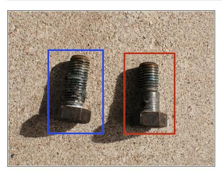
An important note - if you are removing and replacing the front and rear calipers at the same time be sure to keep the front and rear bolts separate.
