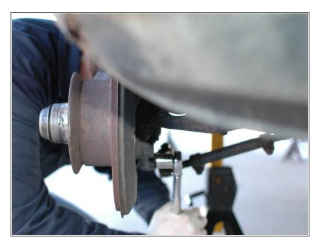
Switch your 19mm socket to a large 1/2 inch drive torque wrench.
