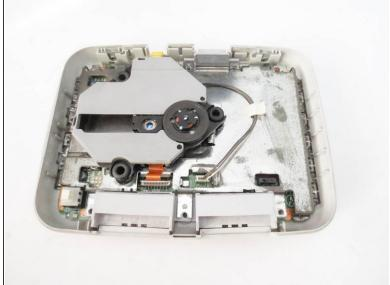
Lift up and remove the upper case.
