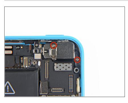
Remove the two 1.5 mm Phillips #000 screws securing the rearfacing camera to the rear case.
