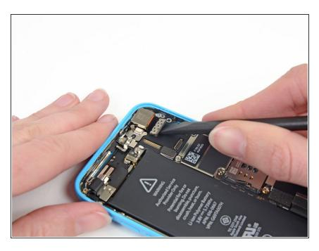
Use the flat edge of a spudger to pry the rear-camera connector up off the logic board.
