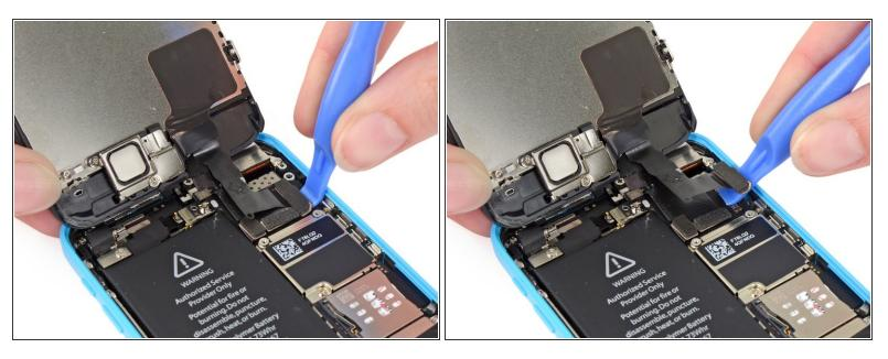
Use a plastic opening tool or a fingernail to disconnect the front-facing camera and sensor cable connector.
