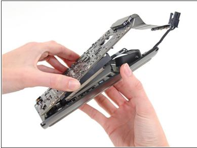
Lift the IO board up from the IO shield from the end with the AC plug.
