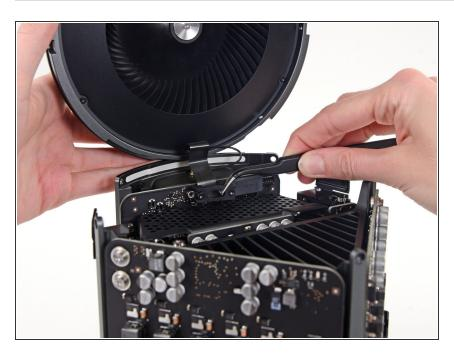
Use a pair of tweezers to pull the fan cable bracket away from the fan assembly.
