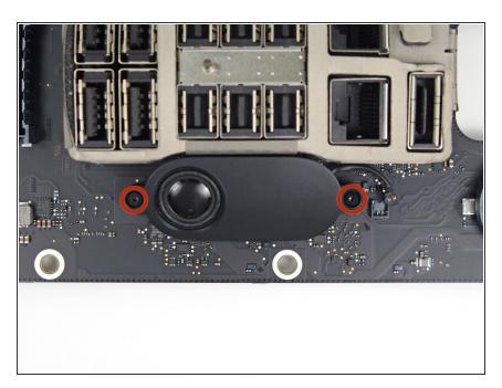
Remove the two 3.2 mm T4 Torx screws securing the speaker to the IO board.
