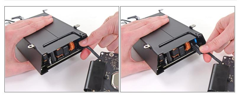
Squeeze the AC power inlet cable connector and pull it straight out of its socket in the power supply.
