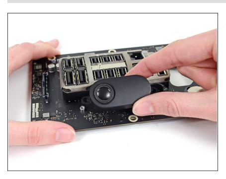
Remove the speaker from the IO board.
