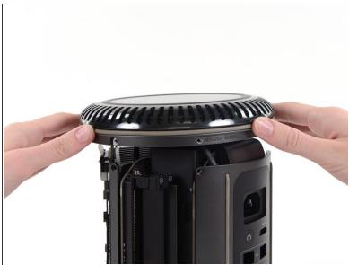
Carefully lift the lower case up and remove it from the Mac Pro.
