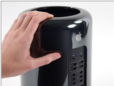
Slide the lock switch to the right, to the unlocked position.
