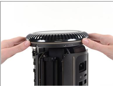
Carefully lift the lower case up and remove it from the Mac Pro.
