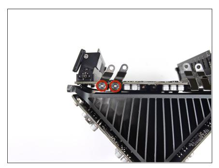
Remove two 5.5 mm T8 Torx screws.
