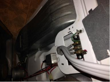
• After removing all screws gently remove the rear cover and cord cover, place them against a wall. Be careful the edges of these can be sharp!
