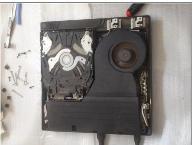
Test the console before assembling. And don't forget to put the spindle disc magnet.
