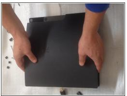
Disconnect all cables. You have 4x Torx T8 screws and 7x Phillips screws. Now you can remove outer case.
