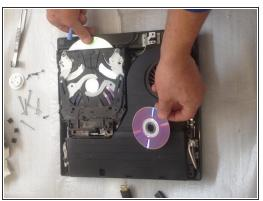
• First remove the spindle disc magnet. Now use plastic tool and slowly extrude the disk from inside.
