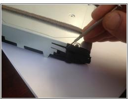
Unscrew the three screws. To remove Blu Ray unit shell you must open two plates that are on the left and right side.
