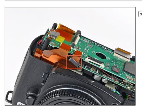
Be sure not to lose the small iron core around the DC-In ribbon cable.
