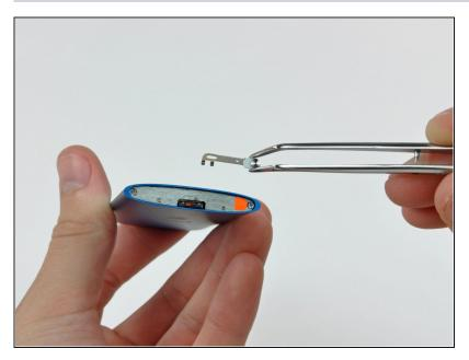
Remove the hold switch slider from the top of the Nano.
