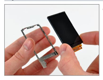
Remove the display from the display bracket.
