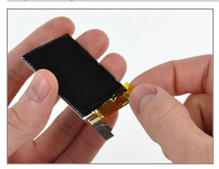
If present, remove the strip of tape covering the display electronics.
