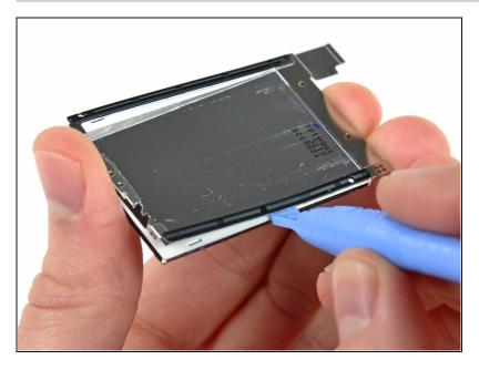
Separate the display bracket from the other side of the display.
