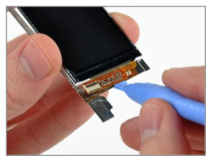
Use an iPod opening tool to carefully peel the display electronics off the display bracket.
