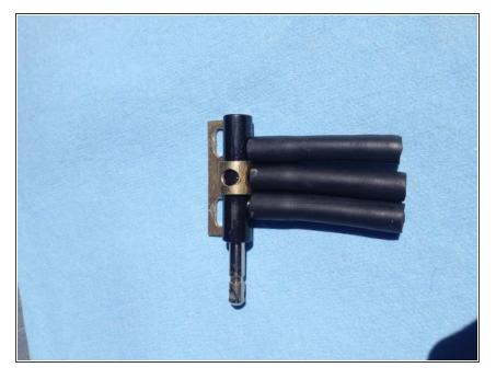
Shown is the vacuum switch removed from the door, with the flexible rubber vacuum connectors still attached. The rubber vacuum connectors may also be left on the plastic hard lines in the door, its your choice.
