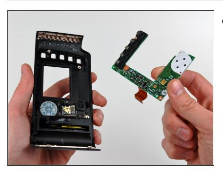
Remove the LCD board from the rear cover.
