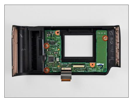
Remove the three 3.1 mm Phillips screws securing the LCD board to the rear cover.
