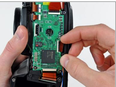
Use your fingernail to flip up the ZIF locking flap on the LCD ribbon cable socket.
