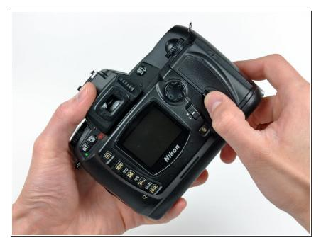
Open the memory door by pushing the memory door retainer away from the LCD.
