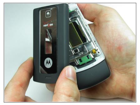
• If the casing has not popped off of the body, remove it carefully from the the phone.
