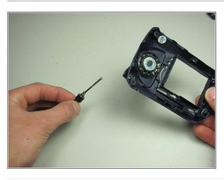
The bad antenna is now removed and may be replaced.
