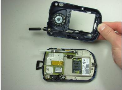
Pry open back plate using spudger.
