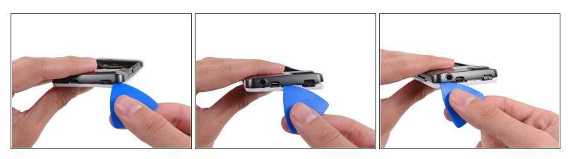
Run the opening pick and pry along the top seam.
