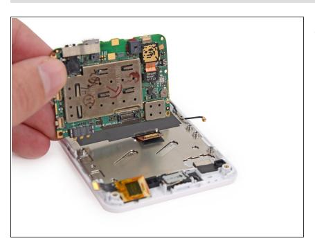
Remove the motherboard from the display assembly.
