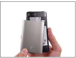
Slide the back cover down and remove it from the phone.
