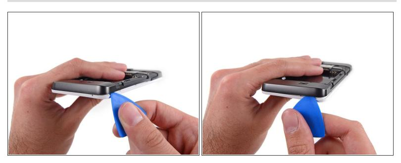
Carefully round the corner, separating the midframe from the display assembly.
