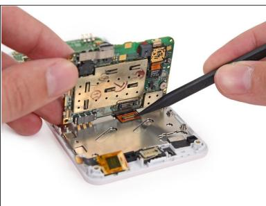
Use the tip of a spudger to disconnect the display data cable from the back of the motherboard.
