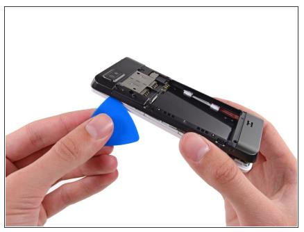
(i) After rounding the next corner, the midframe should be free along the bottom and the sides.
