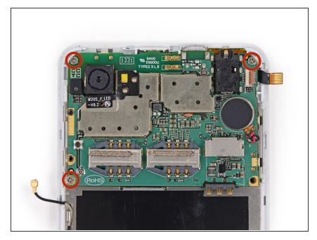
Remove the three 2.5 mm Phillips #000 screws securing the motherboard to the display assembly.
